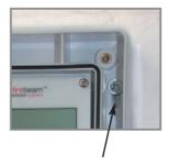
screw in through holes provided out side of the rubber seal
