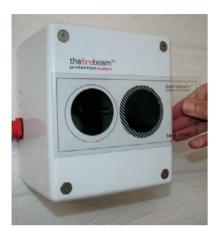
place the filter provided over the eyes of the firebeam
